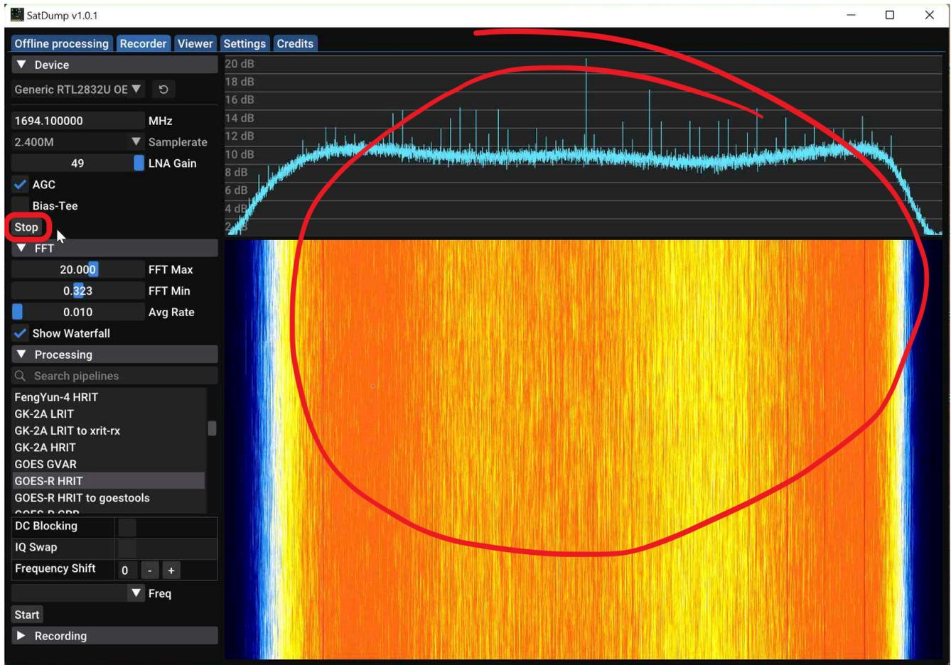
One more time, make sure LNA Gain is slid up or check the AGC checkbox. This is necessary when receiving GOES Weather satellite images. Also, try not to go below 2.048MSPS as a sampling rate for your NESDR device since you will be looking at a relatively wide bandwidth for this application.
