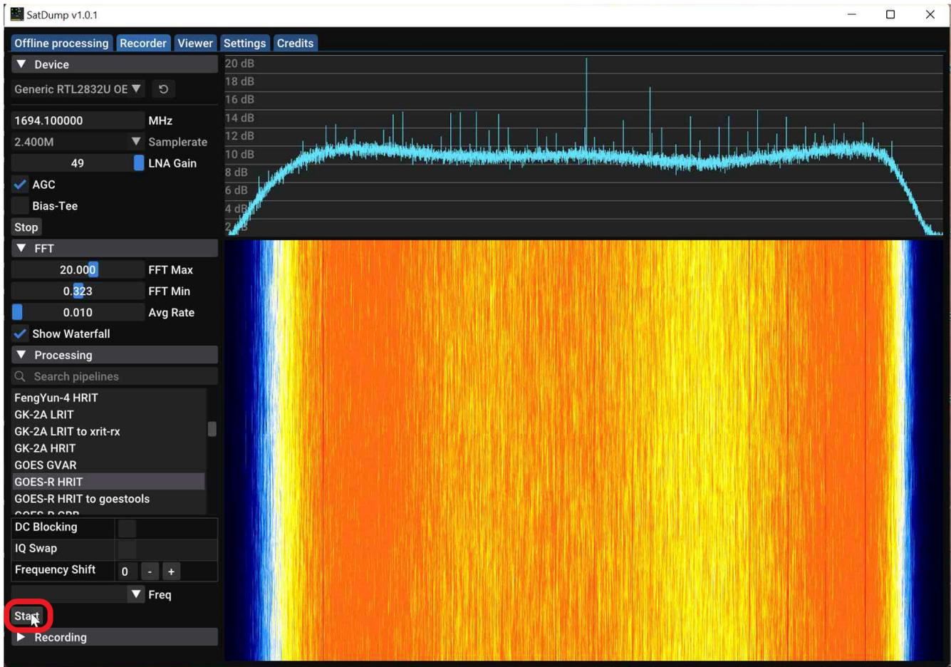
Now navigate to the bottom of the "Processing" tree and hit the "start". This will start the decoding process. You need to make sure you have enough SNR (~6dB and more) for good reception. Below is an example of how SatDump looks without a proper GOES signal fed into the NESDR device.
